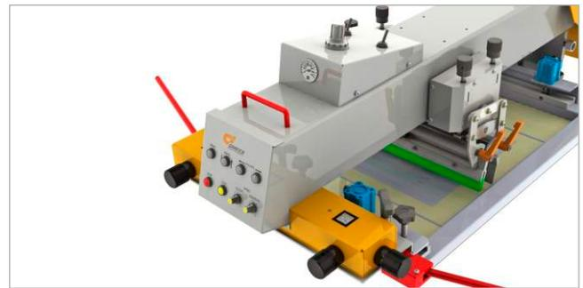
Independent off-contact setting of screen for all four corners and 4-point registration system with safety bar on each head
