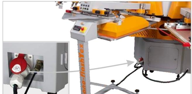
Quick tool free print head lifting mechanism to easily position flash curing unit and in-built electrical ports to connect flash curing unit
