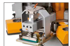
3-point screen registration system and quick-fixing squeegee & flood coater
